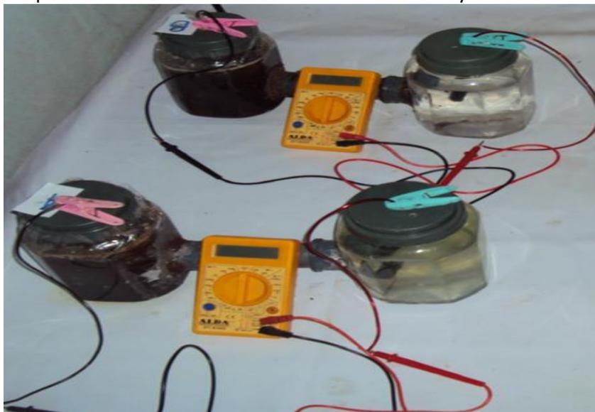
Figure 1. H-shaped (dual Chamber) Microbial Fuel Cell set up.
